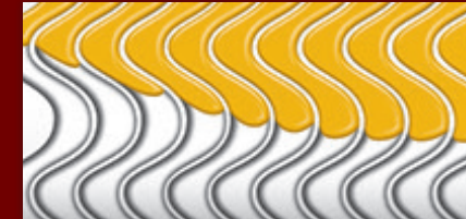
GTT slalom channels reduce ink stress at the doctoring phase for a more controlled ink-to-plate transfer.
