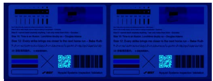
With the UV lighting, the QR code is made clearly visible for inspection
