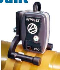
**Document Plate Wear And Damage While the Plate Is Still On Press.** The Betaflex Pro Sensor Head attaches to the Roll Mount, stabilizing the sensor on a stationary plate cylinder for 3D mode measurements. Web print samples can also be imaged on a stationary web over a turning bar or flat area on the press.
