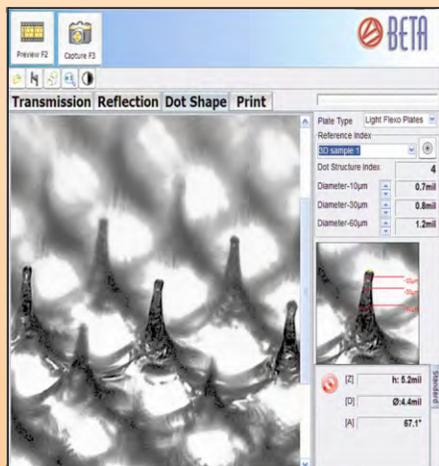
**3D Imaging is the Only Way to Calibrate and Control HD Screening Techniques.** Photopolymer and elastomer plates are easily imaged, analyzed, and compared to the shop standard. "Dot Structure Index" simplifies the production worker's job while detailed measurement data is available to the QC manager.
