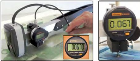
Measure plate gauge, relief of thermal, aqueous, solvent, and direct ablation plates with **FlexiGage Digital Micrometers** to add the data directly to FlexoEye Plus Software ISO database software, see below. The Betaflex Pro Sensor (Measuring Head) and FlexiGage Micrometer can also be mounted on the Sleeve Adaptor or XXL Long Arm System. The **FlexiGage Micrometer** can also be mounted on your existing plate table.
