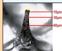
Using reflection illumination, plates are analyzed before or after mounting, flat on the bench, or mounted on the press. Plate wear and damage can now be evaluated before committing to running potentially bad plates.
