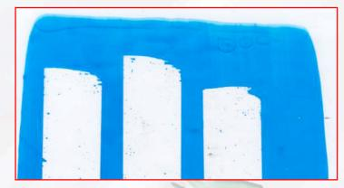
Peeling test on Sun Chemical Pluri-Euro series ink, applied without adhesion promoter, after **CORONA TREATMENT** and oven drying for 10" at 70°C.
