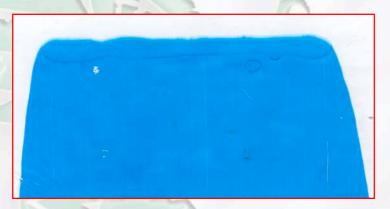
Peeling test on Sun Chemical Pluri-Euro series ink, applied without adhesion promoter, after **FLAME TREATMENT** and oven drying for 10" at 70°C.
